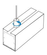
Slide the suspension kits botto mjoiner into the alu base and rotate the joiner until locked into place
