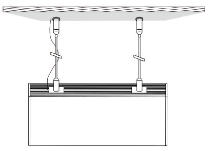
Fix the top joiner to the ceiling. Adjust the cable length to suit
