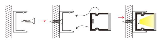
2, Stick the led strip with 3M tape to the flat bar. Put the aluminum flat bar to the led profile directly.
