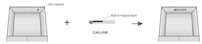
② Be installed on non-iron materials, with double sided adhesive tape.
