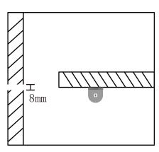
Drill a  $\phi$ 8mm(recommendatory) hole in the backside of the furniture, to allow power supply cable to go through.
