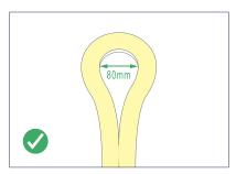
Face to the light surface, fold the strip, the minimum bending diameter is 80mm.
