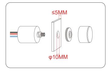
Disassemble the controller and pass through the board in the ways shown above, use a rotating nut to fix the controller, and then press the adjusting knob onto the controller metal rod.
