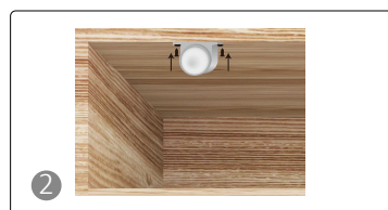
2. Place the sensor in the selected position Then tighten the screws
