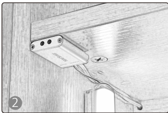
Fixed the sensor onto the cabinet
