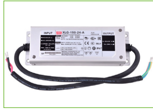
Order code: XLG-150-24-AB AC100-240V DC24V 150W IP67, Global certification 3in1 dimming function: 0-10Vdc, 10V PWM signal and resistance.
