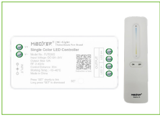
Model: FUT036S+C3 Dimmer: 1 Channel DC12V/24V, 6A, Dimmer, RF remote with finger touch ring.
