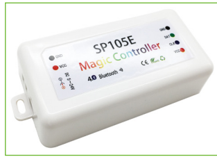
Model: SP105E RGB+IC Controller DC12V/24V Bluetooth APP Control
